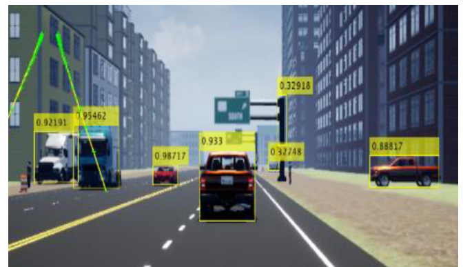
Figure 6. View of the YOLOv2 interface during real-time object detection in an autonomous vehicle. Source: Adapted from Gheorghie et al., (2024)
