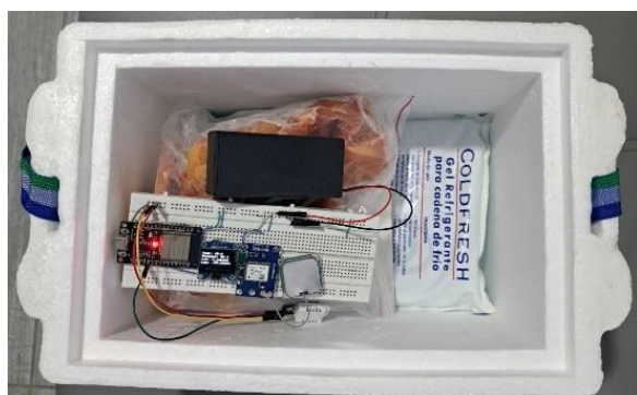
Figure 3. Transport container used for the cold-chain IoT system during land food transportation.
